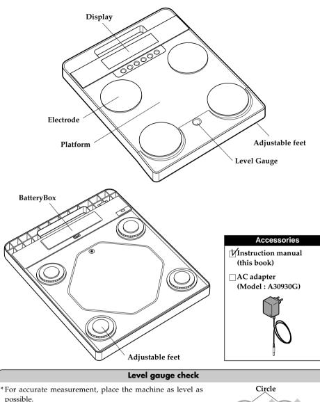
possible. \*Rotate the adjustable feet in 4 positions for adjustment so
